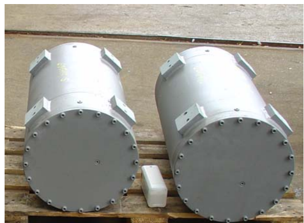
Fig. 33: Transrapid damper of type MTMD-H assembled, integrated in housing and protected against vandalism
