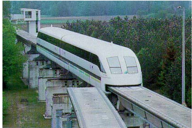
Fig. 30: Transrapid on the elastic steel points girder
