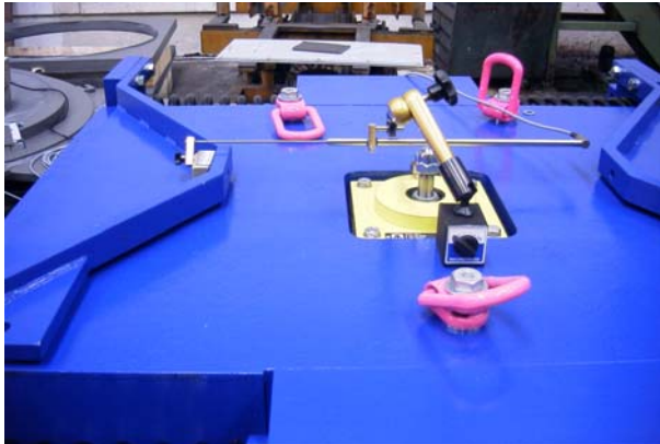
Fig. 52: Testing and possibly fine adjustment of the TMD function characteristics
